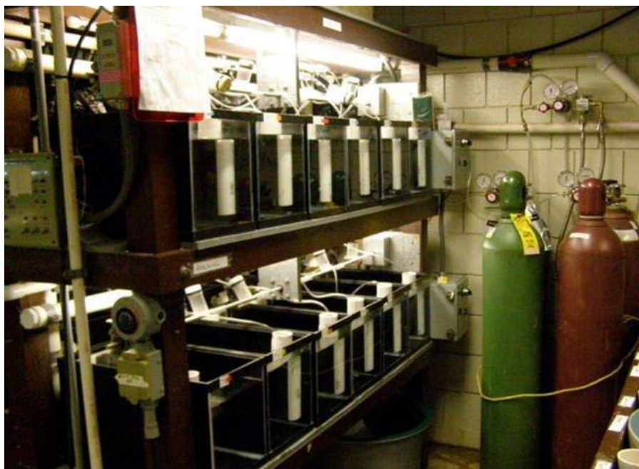
Fig. 1 Picture of the experimental system used during gar and bowfin experiments. Each of the 12 aquariums were equipped with gas-exchange columns to manipulate oxygen level.
