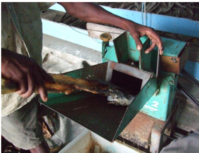
Simple hammer mill for grinding fish carcasses
